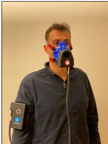
The tool used for metabolic analysis was the Smart Analyzer from DYNOSTICS.
