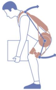
Device ensures user maintains healthy stance when lifting & active force assist (25kgf) supports lumbar muscles
